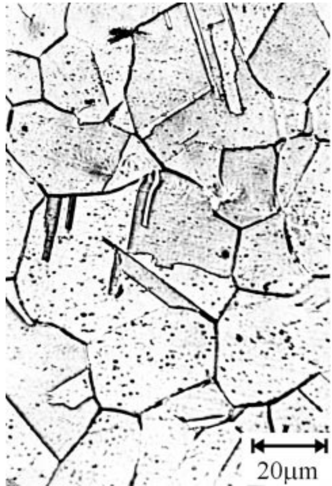
Fig. 2 \kappa -phase precipitation in steel with 4.6 wt.% Al, after aging at 600 °C during 16 h
